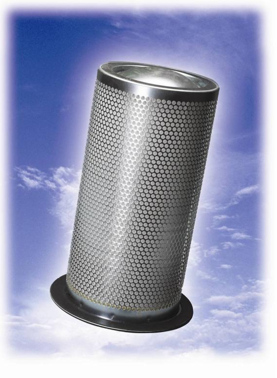
The standard conventional oil separator is the original design for the removal of oil aerosols from the compressed air stream. This element design consists of a specific amount of a uniform grade of borosilicate glass fibers, “wrapped” onto a support tube. When properly sized to the cfm/m<sup>3</sup>/min flowrate and corresponding operating pressure of the machine, this element will provide consistent performance according to the following data:
